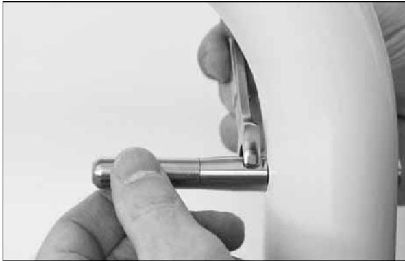
7. Pull the cable tightly along the side of the fitting and mark the cable 1-3/16" from the end of the fitting opposite the post. Mark and cut the cable on your mark.
