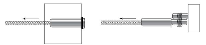
6. Tension the cable with the tensioner installed at the other end of the cable.
