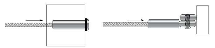
5. Pull cable to set gripping action of the Push-Lock<sup>™</sup> Fitting.
