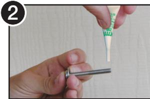
2 Apply a non-permanent thread locking compound to threads.
