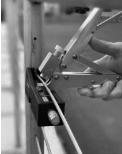
2. Adjust the brass-tip bolt to securely hold the cable. Lock the clamp.
