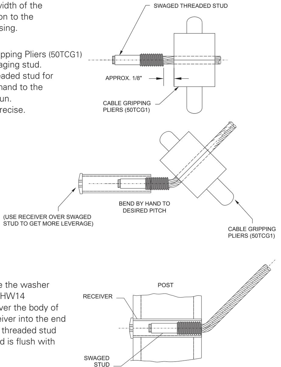
2. Remove the threaded stud. Slide the washer (black plastic for metal posts, 11HW14 stainless steel for wood posts) over the body of the receiver, then install the receiver into the end post. Turn the receiver onto the threaded stud until the end of the threaded stud is flush with the end of the post.
