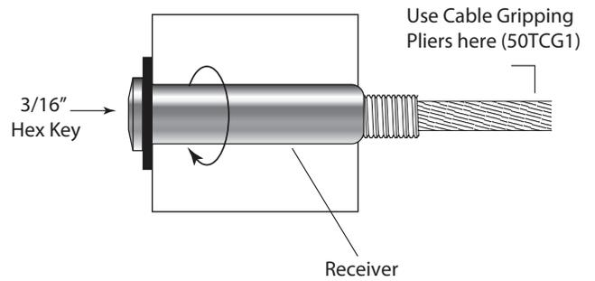
Tension in sequence, beginning with the outside cables and moving from side to side toward the centre
