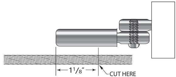
3. Push the cable into the hole in the fitting as far as it will go (approximately 1-1/16"). Twist the cable in the right-hand direction (with the lay of the cable) as you push it into the fitting. You will feel it slide through the jaws inside the stud.
