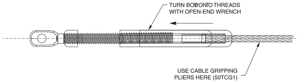
Tension in sequence, beginning with the outside cables and moving from side to side toward the center
