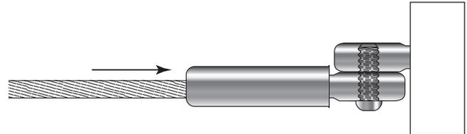
4. Pull the cable, to set the gripping action of the Push-Lock™ fitting.
