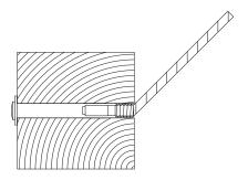
Invisiware® Receivers are less expensive than fittings with fork or eye ends and do not require lag eyes and screws to mount them. When installed, they are hidden inside the end post to help preserve that special view. 20F4062 Invisiware® Receivers are especially designed for 4x4 wood posts and can be an excellent choice for stairs and slopes as well as straight runs.
