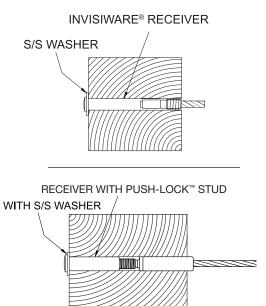
Note: With the Invisiware® Receiver or Receiver with Push-Lock™ stud tensioner, you will need up to 3-3/4" of space between the back of your end post and any structure to insert the fitting into the end post from the back side.
