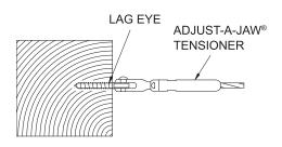
The other end of each cable run can be either a tensioner (above) or a non-tensioning device. Following are **non-tensioning devices.**
