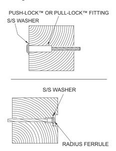
Note: With the Radius Ferrule, Push-Lock™ or Pull-Lock™ fittings, you will need approximately 2-1/2" of space between the back of your end post and any structure to insert the fitting into the end post from the back side.
