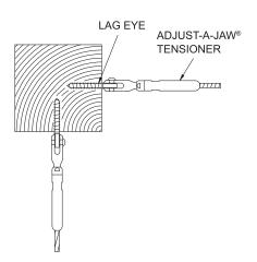
d) Hardware used for stairs or severe slopes. You can use any of the fittings with a fork or an eye in conjunction with a Lag Eye, to accommodate stairs and slopes. These fittings are Adjust-A-Jaw<sup>®</sup>, Adjust-A-Body<sup>®</sup> with Threaded Eye tensioners, Fixed Jaw and Push-Lock<sup>™</sup> with threaded eye non-tensioning fittings.
