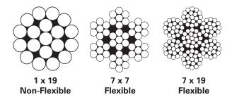
You will want to specify type 316 stainless steel, because it is the most corrosion resistant commercially available alloy used in manufacturing cable. Cable Art hardware is made from type 316 stainless steel, so no material compatibility issues will arise when you use type 316 stainless steel cable with Cable Art hardware.
