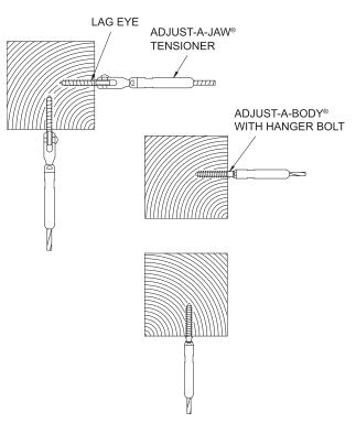
A corner may be designed using two posts on the corner and running the cables between the posts as illustrated below. There must be a tensioner on both ends.
