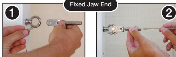
1 Install eyebolt. Remove clevis pin and install Quick-Connect® Fixed Jaw fitting.
