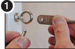
1 Install Jaw onto an eyebolt or eyelet using the removable clevis pin.
