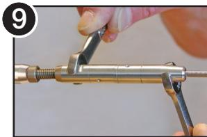
9 Use 3/8" wrenches to tighten the Quick-Connect® to desired final tension.
