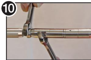
10 Tighten the lock-nut against the Quick-Connect® to prevent the fitting from loosening.
