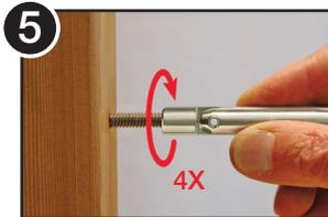
5 Attach the pivot end of the Quick-Connect® and rotate the body 4 full turns.
