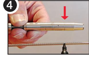
4 Stretch cable tight across fitting and mark at Cut Gauge Line. Cut cable at mark.
