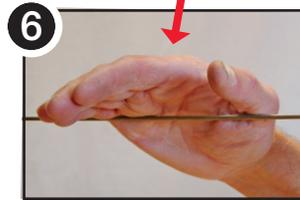
6 Hand tighten the Quick-Connect® as far as possible, then swiftly hit the cable line with your palm several times to ensure that jaws are securely seated.
